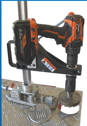
Drilling aluminium Checker plate with 100mm holesaw
