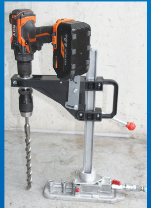
Long series drill up to 360mm long.
