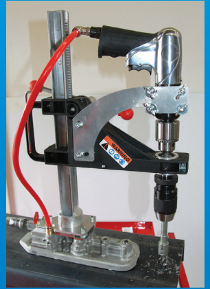
Air supplied from safety valve, which delivers air only when the vacuum plate is fixed.
