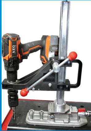
Thread Tapping up to 16mm
